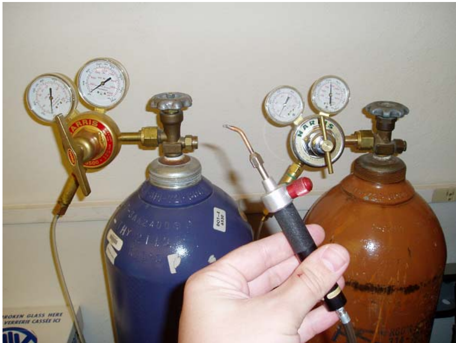
Figure A.7: H 2 /O 2 cylinders and torch
