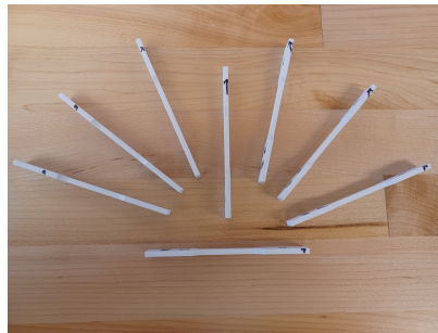
(b) Specimens printed in the horizontal orientation and at eight print bed angles after removal from the print bed.
