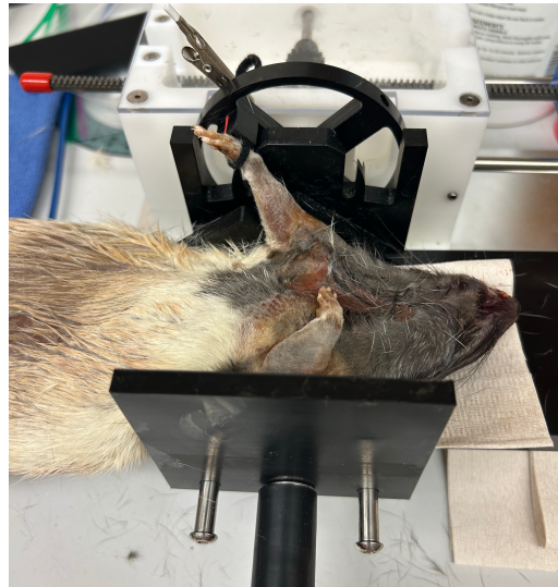
Figure 5: Rat in RatFlex device with riser in place. Ramp is offset with the original ramp. These changes did yield more consistent results. Shown below are some of the graphs after the changes were made to the device.
