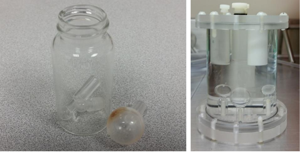
Figure 37 Thin-wall hot-spot spheres (diameter = 7.7, 9.8, 15.8 mm) placed in a cylindrical phantom of ~10 cm in diameter.
