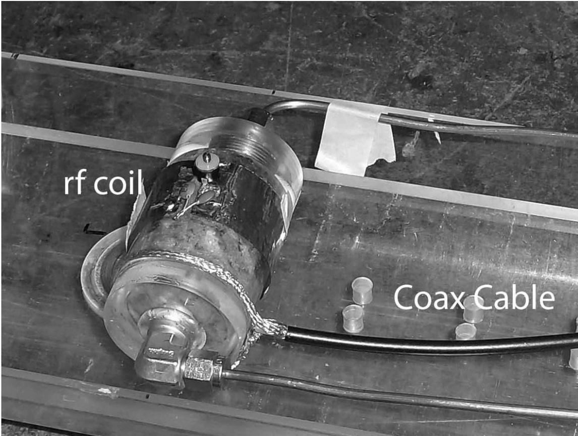
Figure B.1. Lung sample in cylinder with rf coil. This is the coil for helium. The two 22 pf capacitors in series and the variable capacitor can be seen on the top of the rf coil
