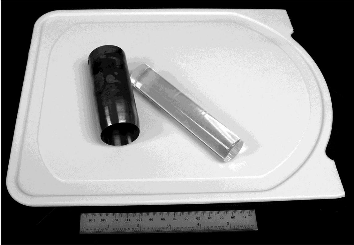
Figure B.5. The cutting apparatus. The stainless steel meat cutter of 1 3/8 inch diameter (sharp edge facing down in the picture), a plastic cutting board, and plastic cylinder to assist in removing the cut core from the meat cutter. A six inch ruler is placed in the photograph for scale.
