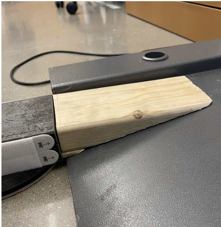
Figure 26: Demonstration of wood wedge offsetting the ramp
