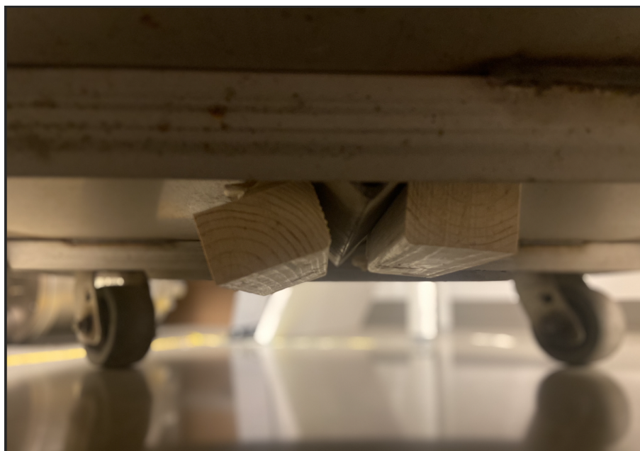
Figure 28: Wooden pieces under tank, creating a flatter surface
