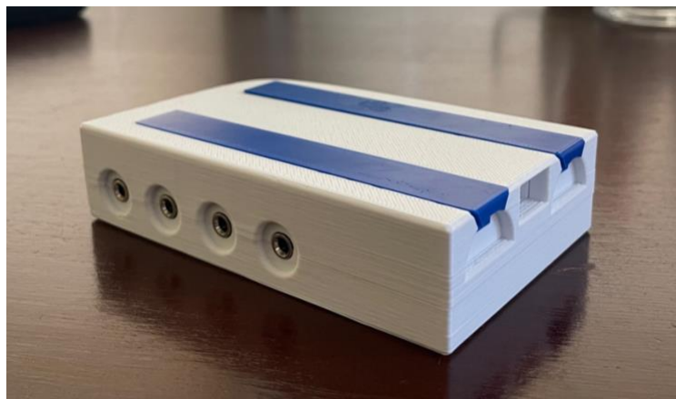
Figure 13C Isometric view of final housing with chip design integrated
