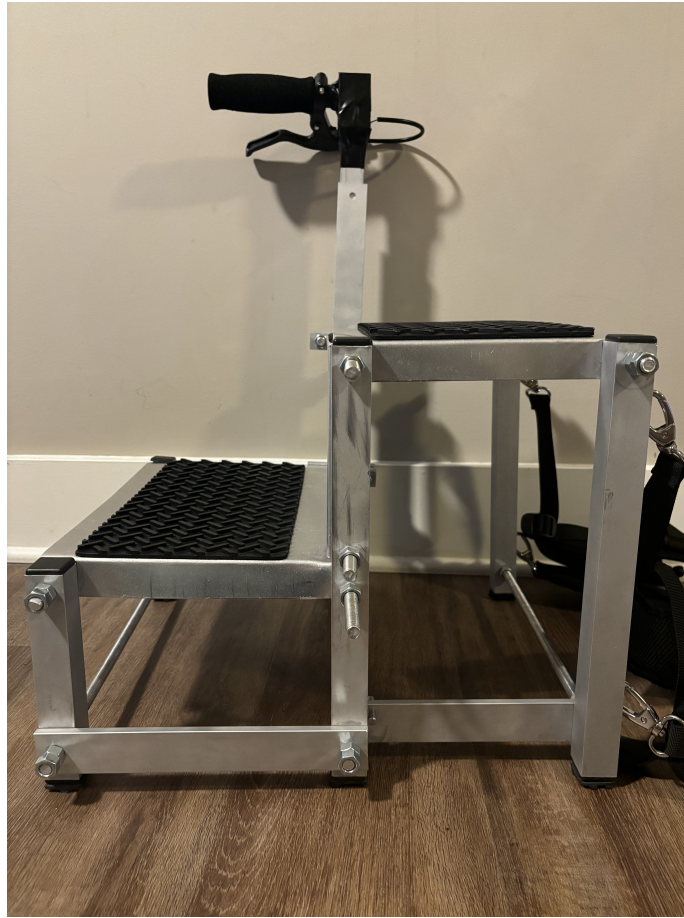
Figure 29: The pin-box mechanism that holds the handle in the expanded position.
