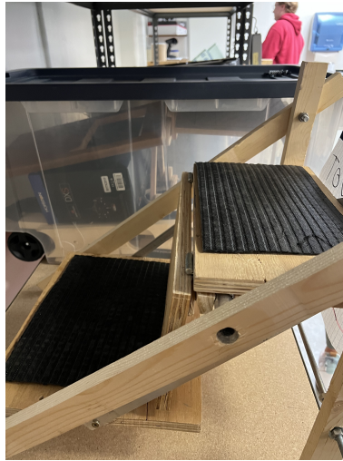
(c) Final Concept Prototype: Includes plastic mats for increased grip when stepping. The beams running across are strong and held in place with hot glue.
