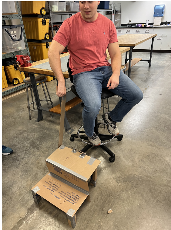
Figure 7: Photo of the mockup prototype created. Benjamin is shown holding the handle while on a high chair, simulating how it would be inside a truck.
