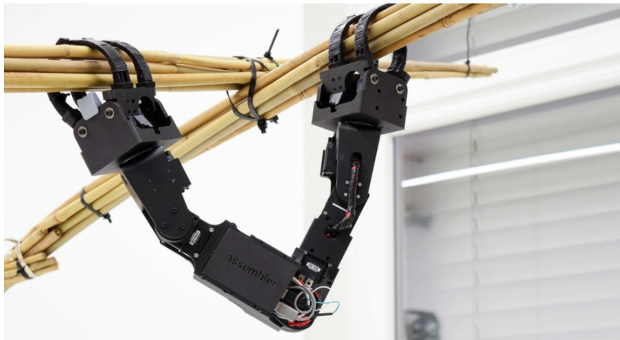
Figure 1: Proposed robot clamping onto bamboo clusters
