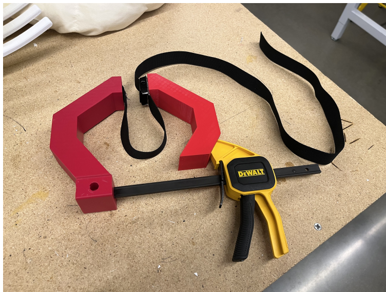
Figure 30: Adapted Trigger Clamp Final Prototype
