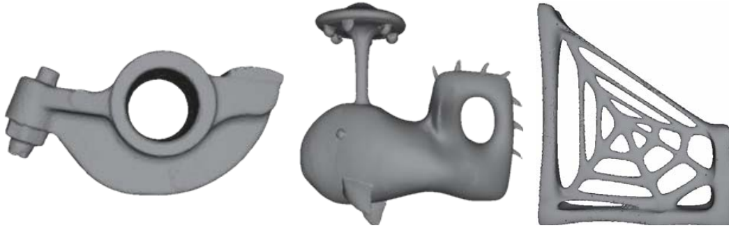
Fig. 16. Using Polymender to produce a water-tight surface from a set of triangles.
