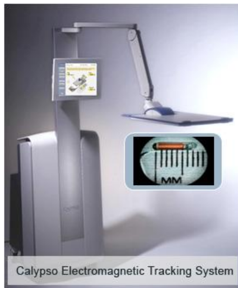
Figure A.1 Calypso electromagnetic tracking array. Inset displays the implantable electromagnetic transponders (Image courtesy of Calypso Medical).
