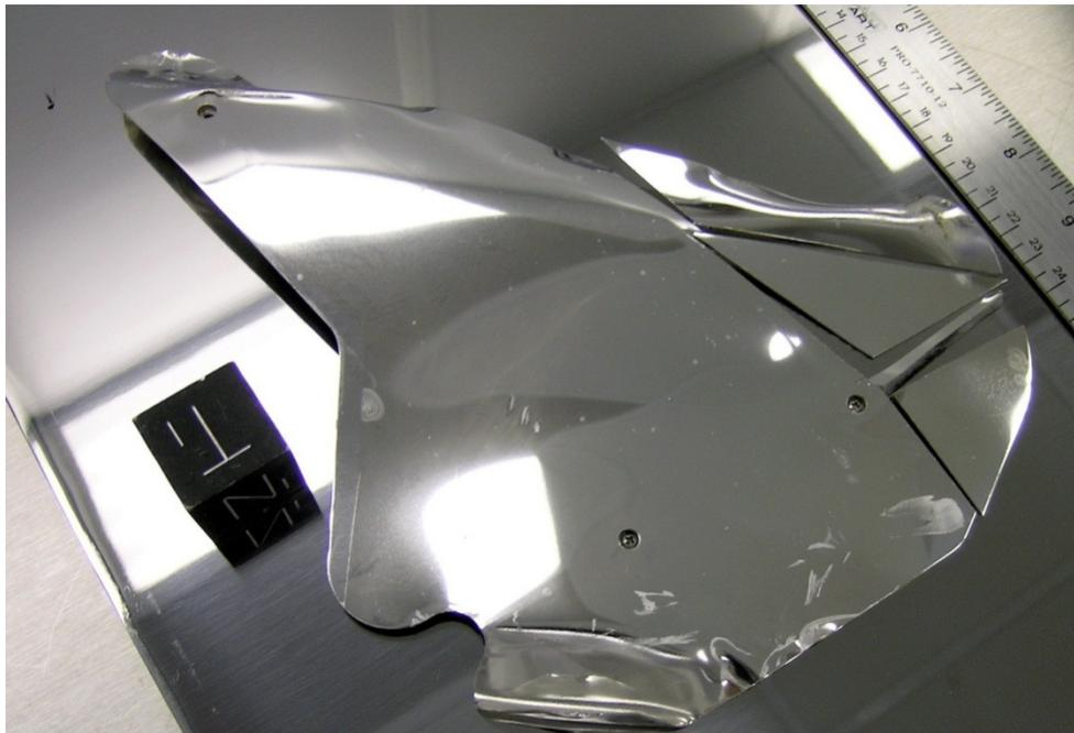
The PAC was made from a standard commercial aluminum alloy #6061-T6, milled to 0.025-inches-thick, and then hand polished at JSC (Allton et al. 2005). The major trace components of the 6061 alloy are Mg, Si, and Fe (Aluminum Association 2000). These change the physical and thermal properties relative to pure Al, which are compared in Table 1.1. Of particular importance for this work, the 6061 alloy has a lower melting temperature than pure Al.
