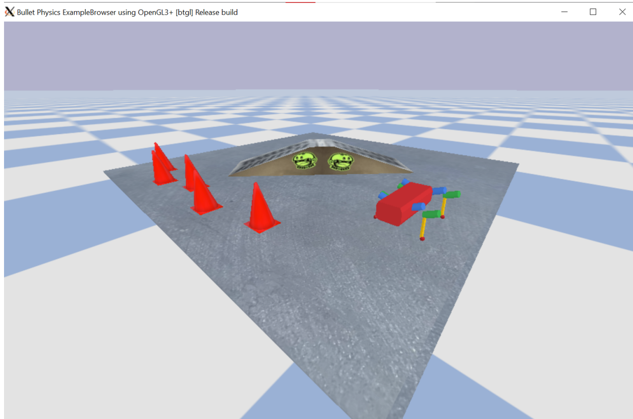
Figure 3. Simulator using PyBullet to recreate the Pupper robot and some additional obstacles
