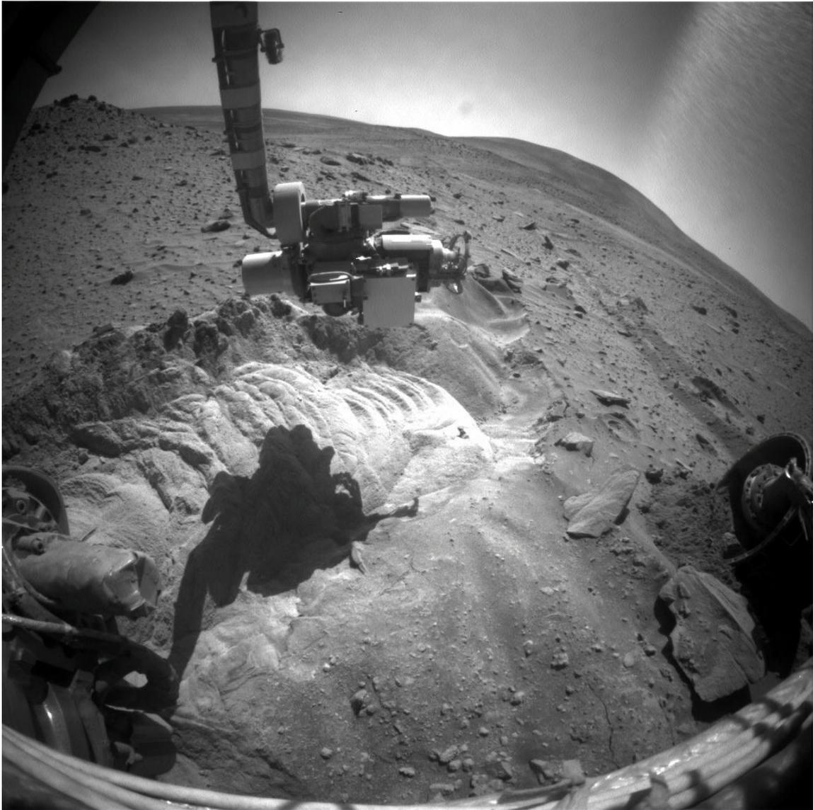
Figure 3.12: Front Hazcam showing the severity of embedding in Troy. The left-front wheel should be visible, but it is completely buried in the trench of high-albedo cohesionless sands. This image was taken on sol 2154.
