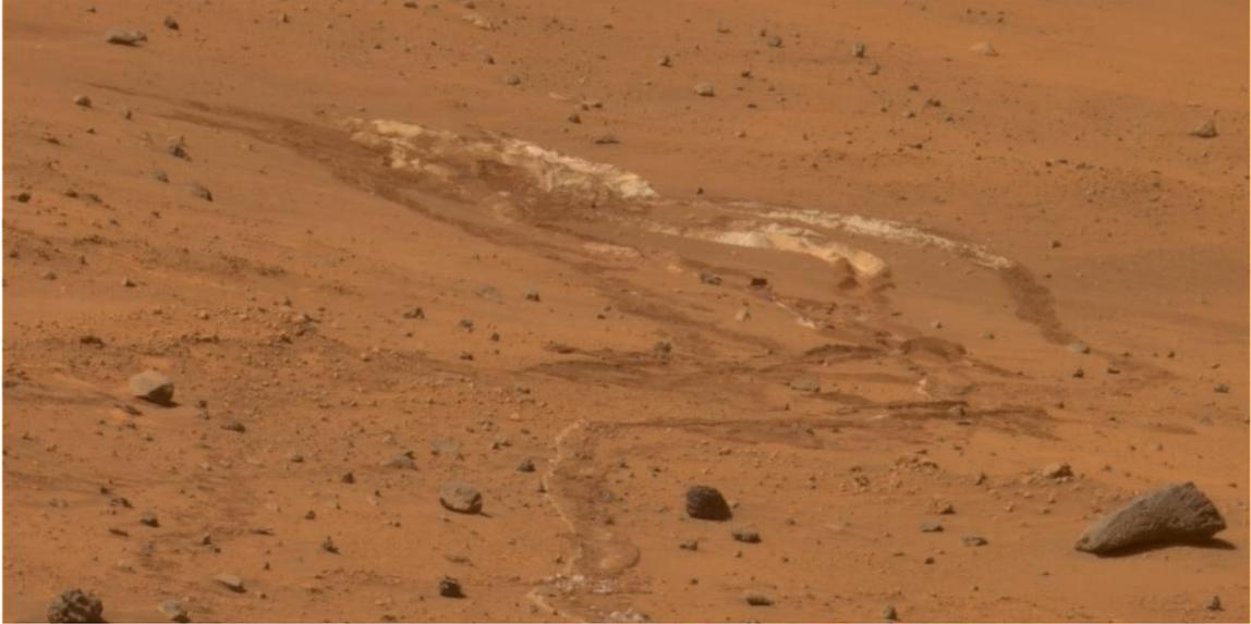
Figure 1.3 Pancam image of Spirit wheel tracks in a poor mobility situation (5 wheels; soft soil). This image was taken on sol 959 looking back at “Tyrone”.
