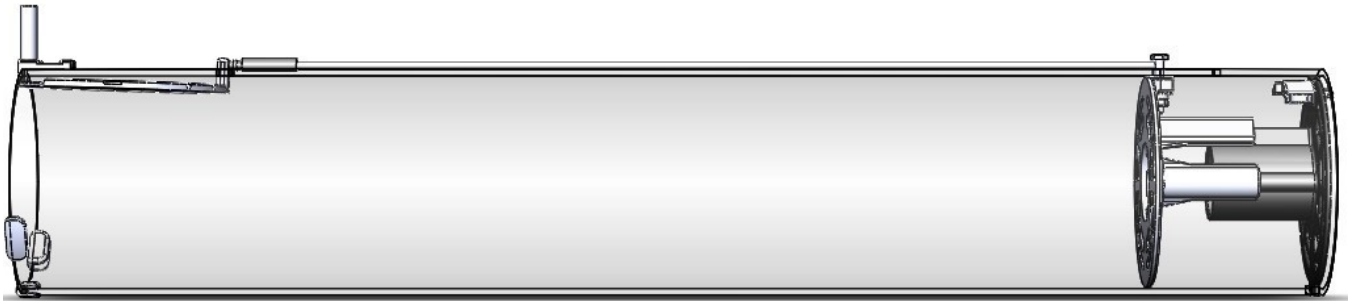
Figure 31: Side view of the Q.T. B-BAR Rat Trap in an opened state. Note how the Dowel Pin is in the door release and the Push Plate is fully extended
