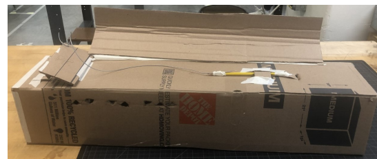
Figure 12: Trap with the lid open showing the trigger-induced pressure pad to close the door to prevent the rat from escaping
