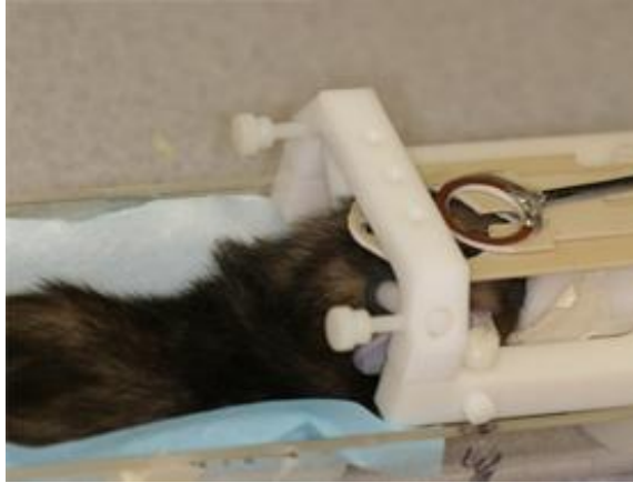
Figure 5.1: MRI-compatible device to hold the head of the ferret still during an experiment. A mixture of isoflourane and oxygen is supplied through the nose cone. A receive surface-coil is placed above the head. The transmit coil (not shown) surrounds the entire setup when placed in the magnet. Image reproduced with permission of author (Barnette et al., 2009).
