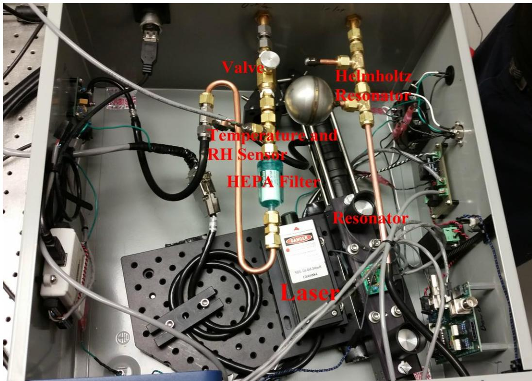
Figure 2.7 View of the resonator installed in the enclosing (assembly) box.
