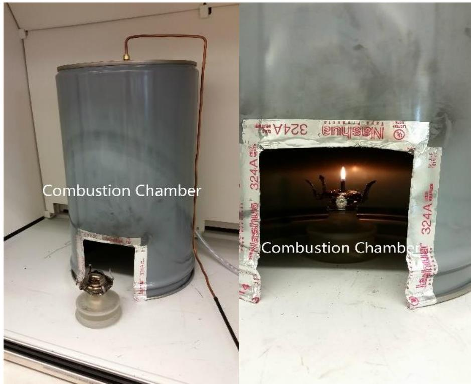
Figure 3.4 The black carbon sub-micron aggregate generator
