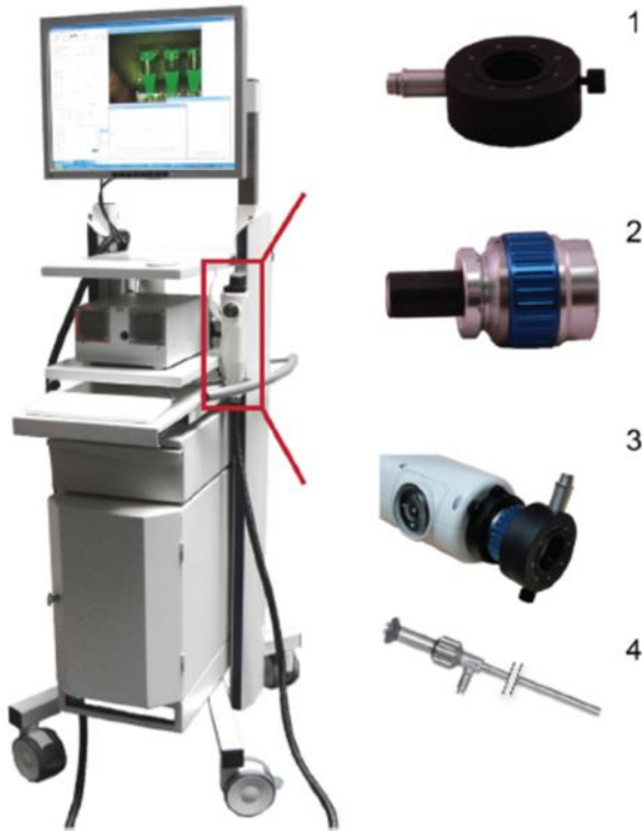
Figure 6: The Quest Spectrum (Artemis) NIR imaging system. The ring light (1) and lens (2) that have to be attached to the handheld camera (3) to obtain NIR fluorescence images. For minimally invasive applications, a scope (4) can be attached to the handheld camera instead. Reproduced with permission. 4
