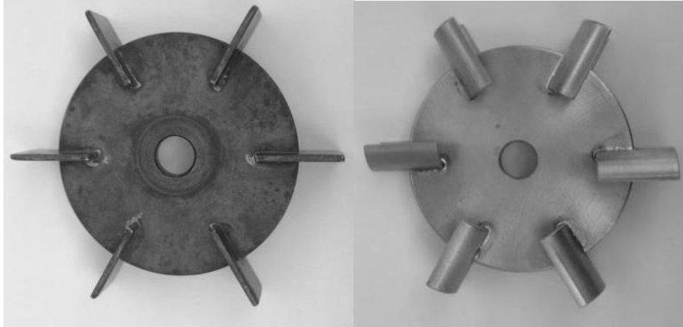
Figure 4.7: Rushton turbine (left) and half circular blades disk impeller (right).
