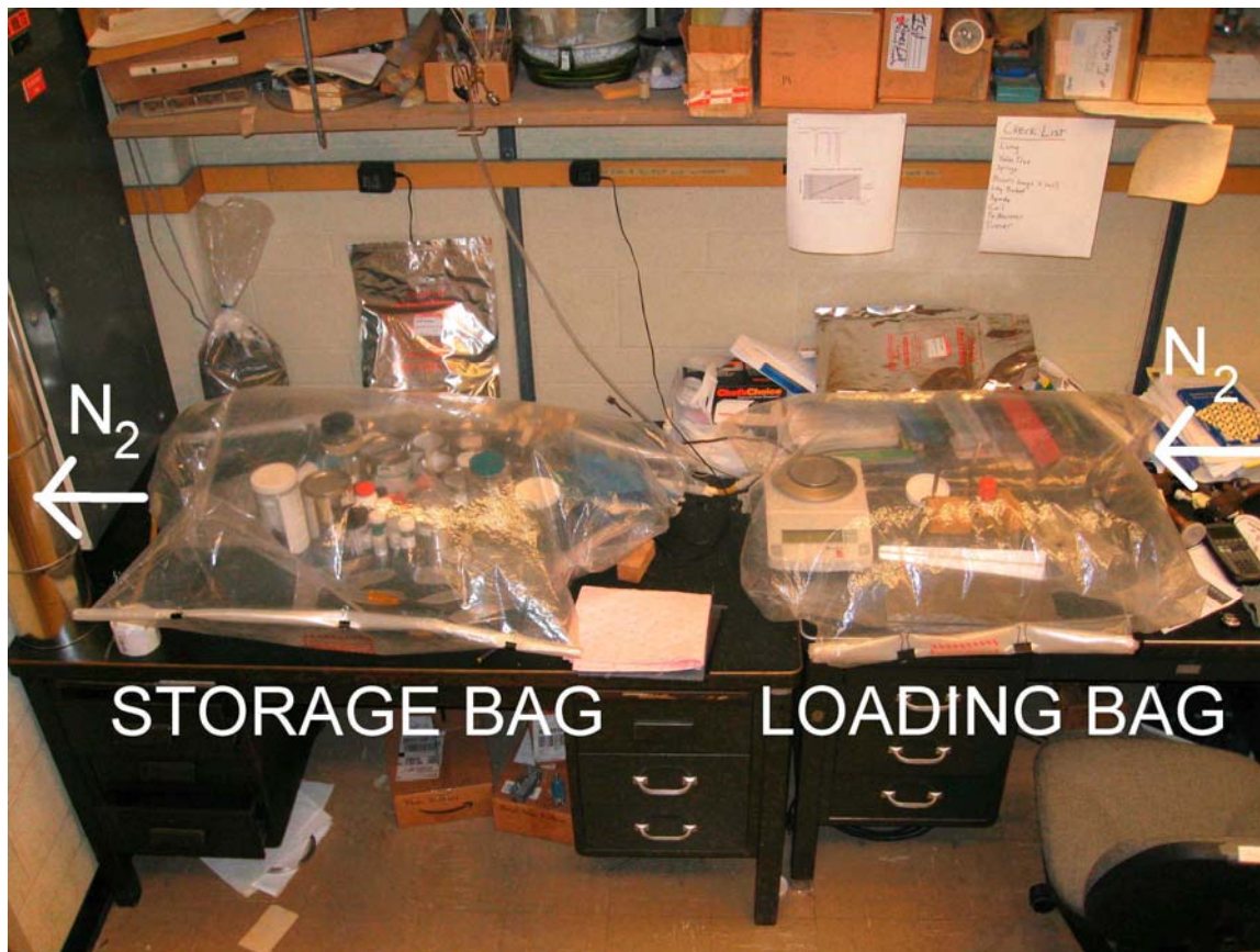
Figure 2.9: Glove bags used for sample manipulation and storage.
