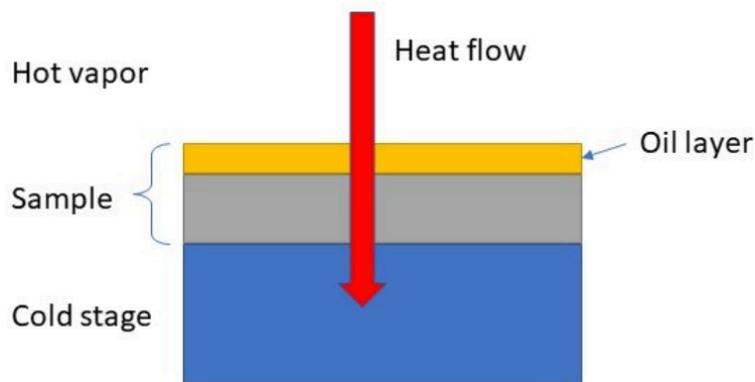
*Figure 1. Schematic of Heat Transfer on Lubricant-Infused Surfaces (LISs)*
