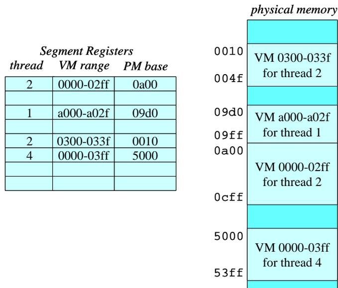
**Figure 6. Segmented VM with pooled segment registers**
