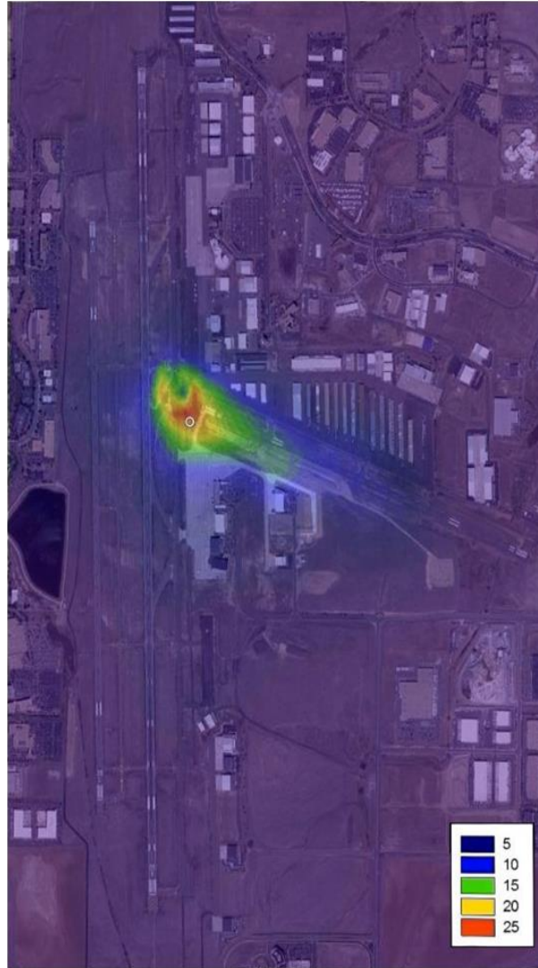
Figure 2-8 Modeled average September lead impacts in \text{ng/m}^3 using the refined model. Background image from Google Earth™.
