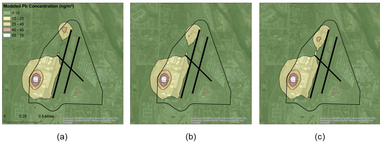
Figure 5-8 Modeled three-month average concentrations from November-January at RVS using the: (a) original runup areas; (b) Z1 runup areas; and (c) Z2 runup areas. The large hotspot in the southwest corner of the footprint is from engine testing emissions.
