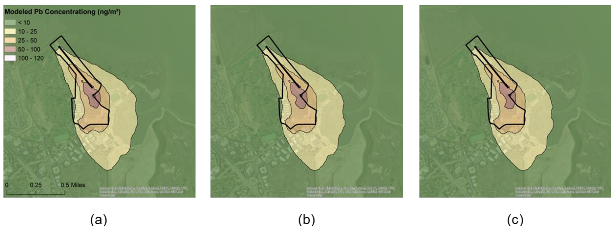
Figure 5-11 Modeled three-month average concentrations from November-January at SMO using the: (a) original runup areas; (b) Z1 runup areas; and (c) Z2 runup areas.
