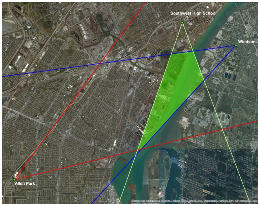
Figure A-1 Triangulation of NWR results for SO 2 monitors in the Detroit area. Analysis performed by Dr. Varun Yadav using hourly data.
