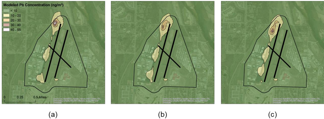
Figure 5-9 Modeled three-month average concentrations from November-January at RVS with engine testing emissions removed using the: (a) original runup areas; (b) Z1 runup areas; and (c) Z2 runup areas. Engine testing emissions were excluded from this analysis.
