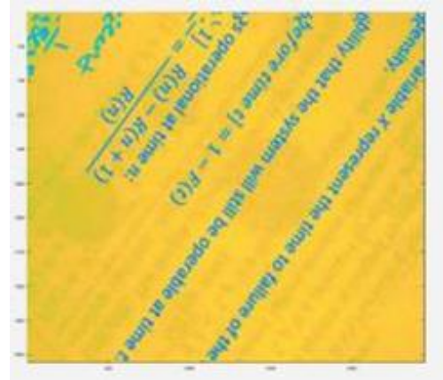
Figure 3. A pseudo-color image created using raw pixel data reconstructed into an image using MATLAB
