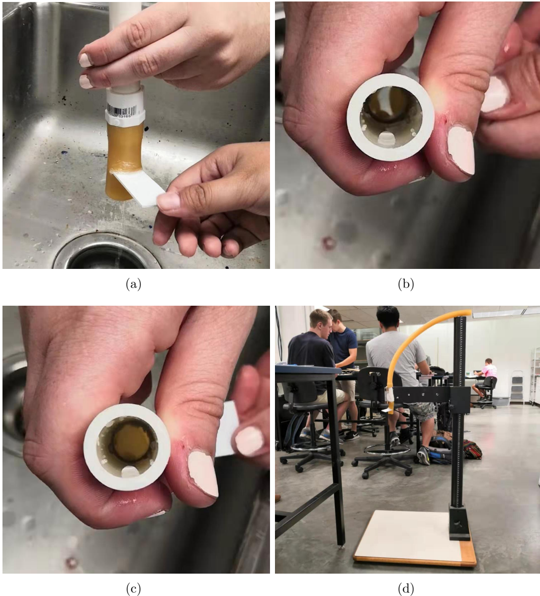
Figure 8: (a)The mockup of tube and nozzle, (b) Top view of tube when the blocker is open, (c) Top view of tube when the blocker is closed, (d) Final mockup with a holder
