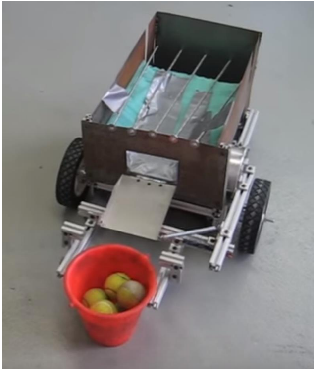
Fig. 2.3 The robotic ball sorter with its two prong and hinging grabber. The grill in the bucket sorts the balls which are released through the door on the front.
