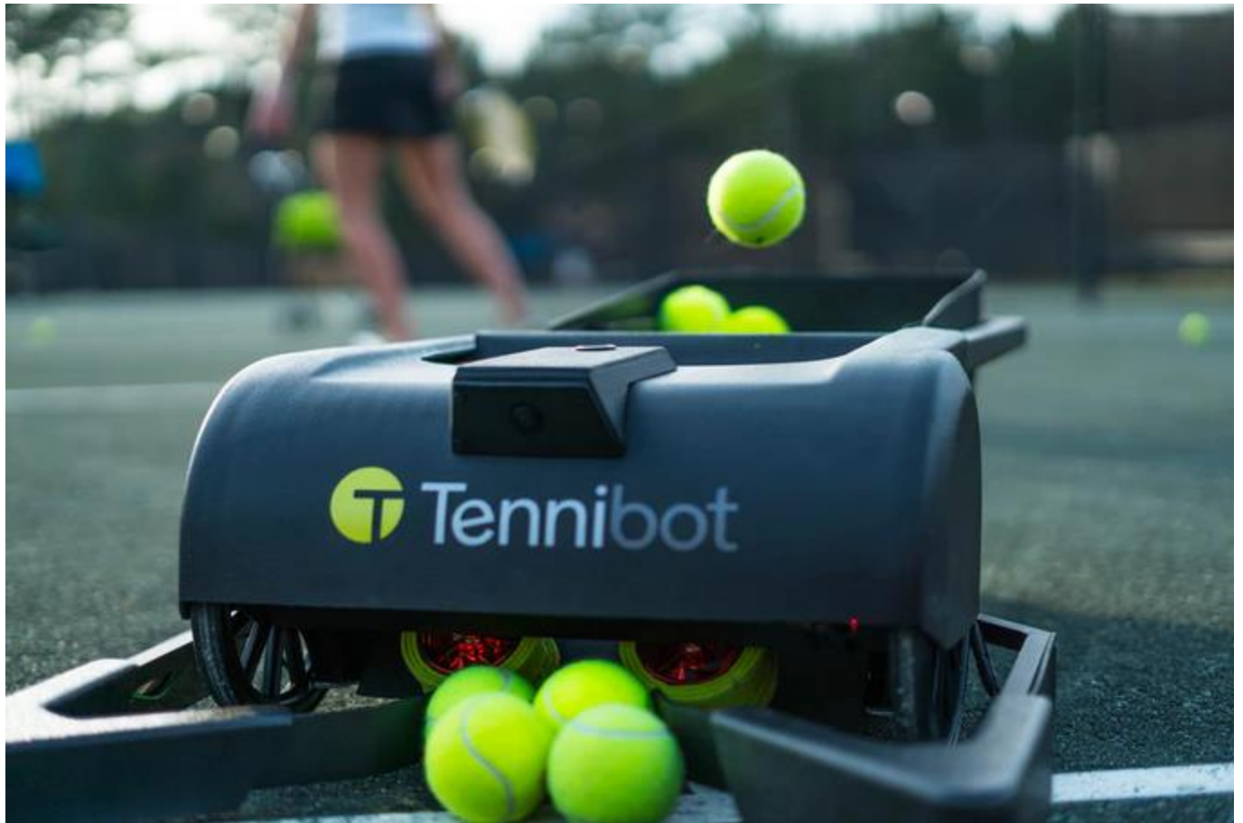
Fig. 2.2 The Tennibot that autonomously navigates a tennis court picking up and storing balls.
