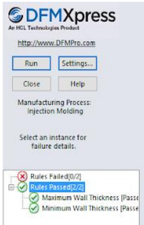
Figure 34: The DFM analysis for injection molding for our designated part
