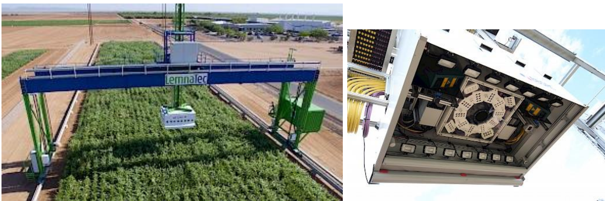
(Source: LemnaTec) Figure 3. Transect FluorCam (Left) Internal imaging system in a weather-proof cabinet (Right)
