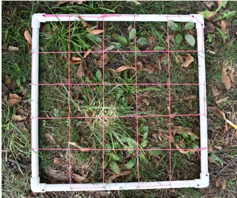
Figure 1. Current 50 x 50 cm PVC rig used to count infected plants by hand.
