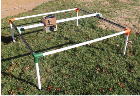
Figure 1. First prototype of an automated small-scale plant imaging system
