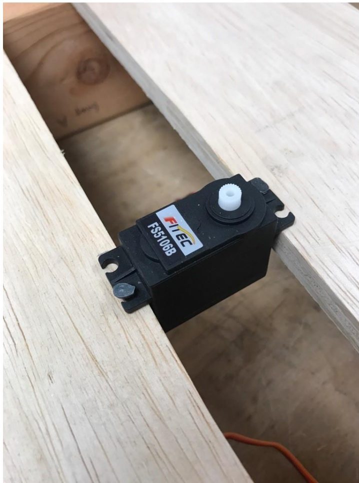
Figure 20: Servo motor mounting to turn rotating base
