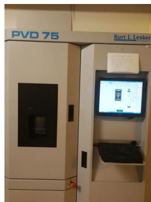
Figure 2.8 Kurt Lesker PVD 75 Physical Vapor Deposition system
