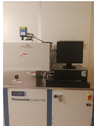
Figure 2.9 Oxford Instrument's Plasmalab System 100 Inductively Coupled Plasma
