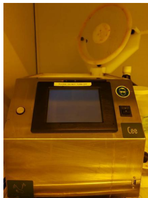
Figure 2.6 Brewer Science CEE 200X Spin Coater.
