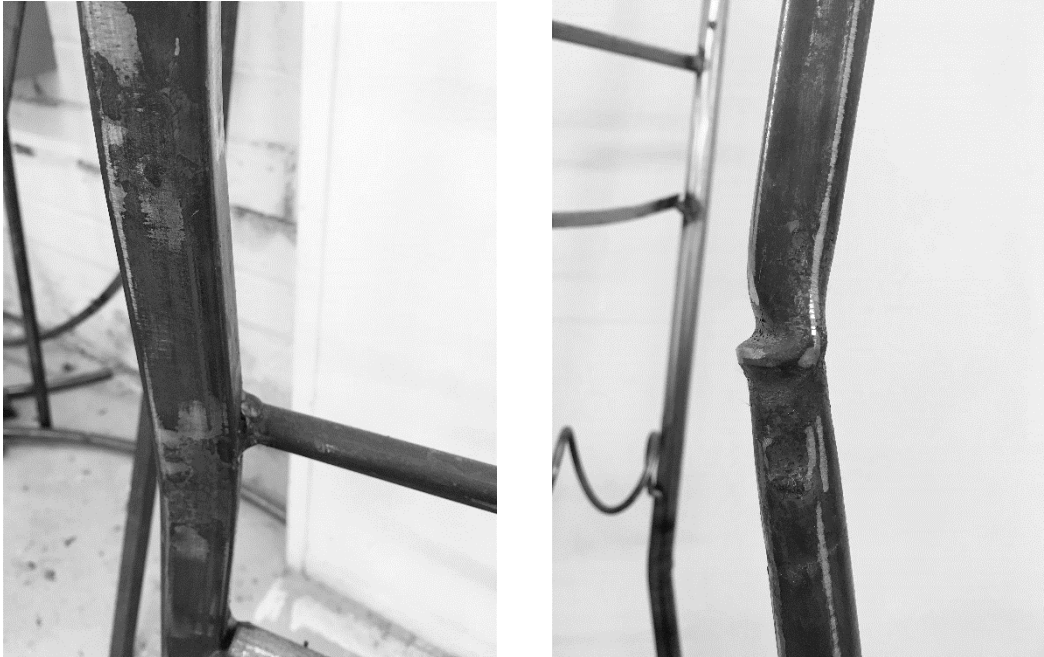
Raw steel process details: welding, heat bending, sanding.
