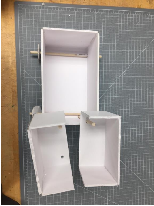
Figure 11: Mockup side view with lowered collector
