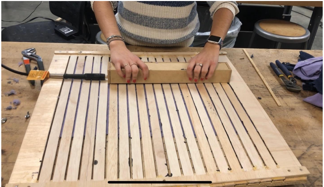
Figure 24 The T-shirt 2 Cutter in use with a purple shirt in between the waffle base and the slotted guide
