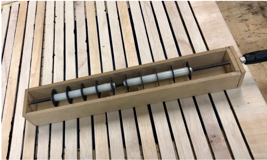
Figure 25 The blade array inside the blade case, resting atop the slotted guide
