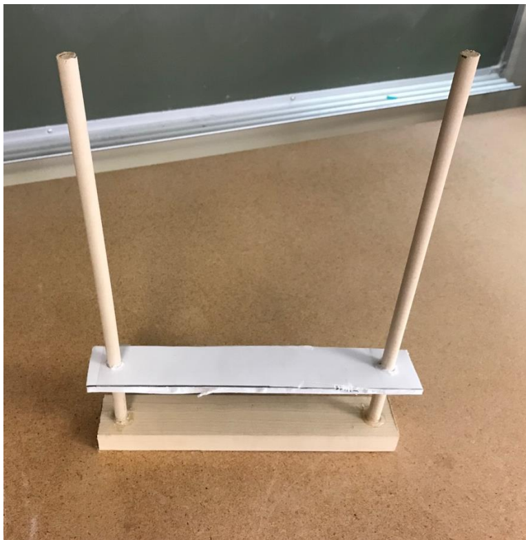
Figure 5. Frontal view of glue joint aide with carriage in lower position
