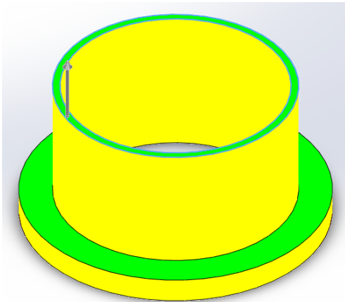
Figure 7-4 Positive draft angle applied to the bushing
