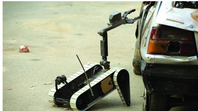
Figure 2-6: SUGV reaching into a car
