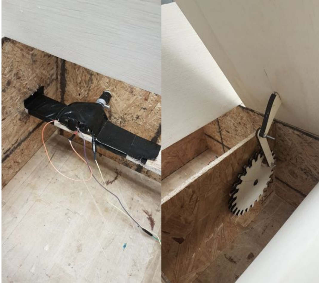
Figure 18 Gear driven by the DC Motor behind for the top board
