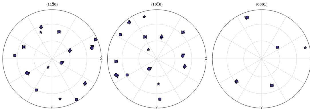
**Figure 9** Orientations of individual quartz grains tested at room temperature. Shapes correspond to points on previous plot.
