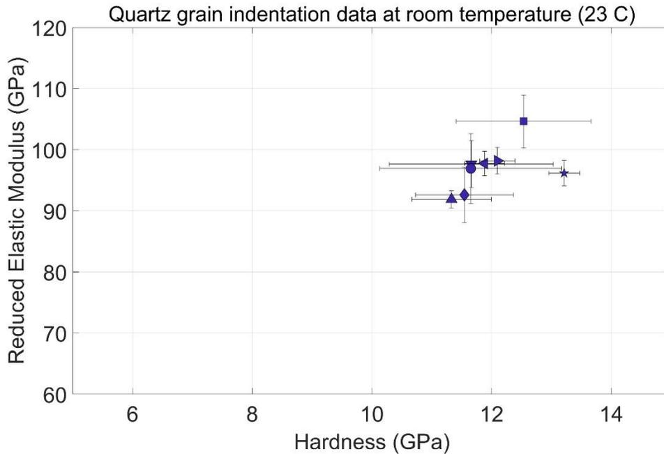
Figure 8 Average elastic modulus vs. average hardness for all quartz grains tested at room temperature.
