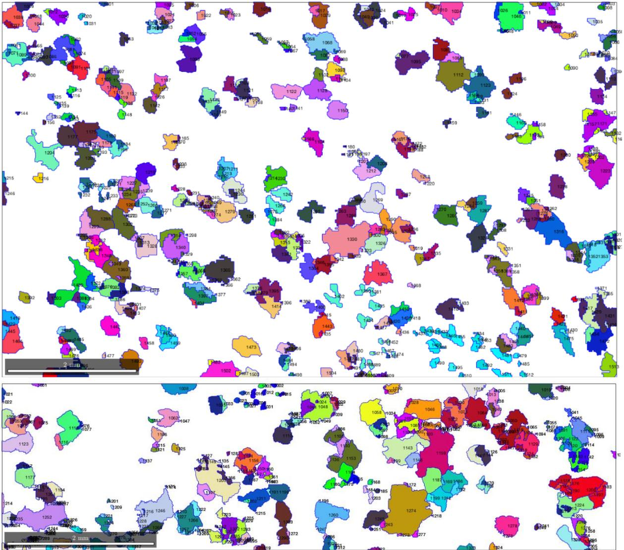
Figure 2 Orientation map of quartz grains within Westerly Granite sample.
