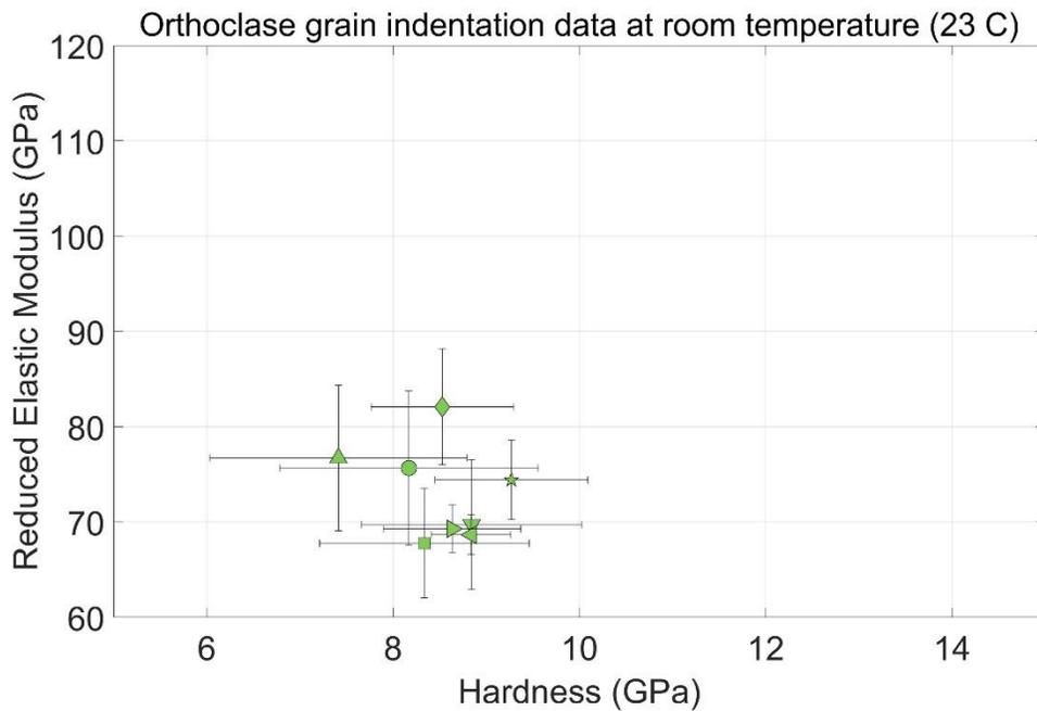
**Figure 12** Average elastic modulus vs. average hardness for all orthoclase grains tested at room temperature.
