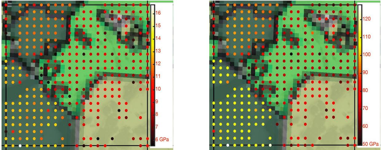
*Figure 5* Hardness (left) and elastic modulus (right) of 21x21 indentation array area with 10  $\mu\text{m}$  spacing.
