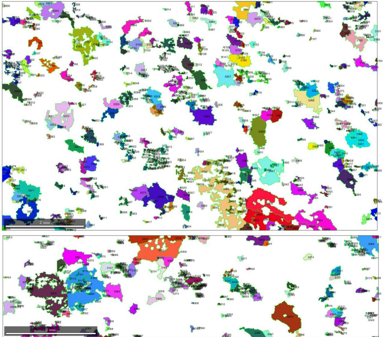
Figure 4 Orientation map of orthoclase grains within Westerly Granite sample.
