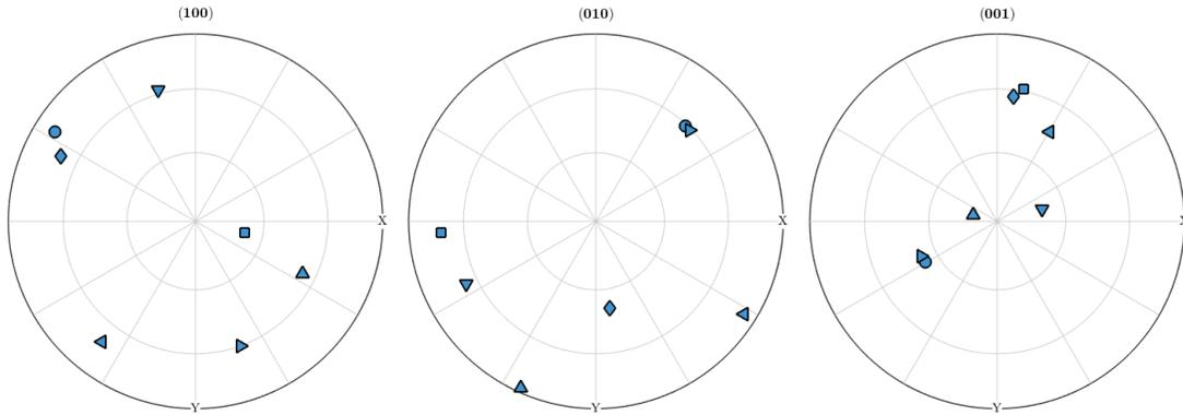
**Figure 11** Orientations of individual plagioclase grains tested at room temperature. Shapes correspond to points on previous plot.
