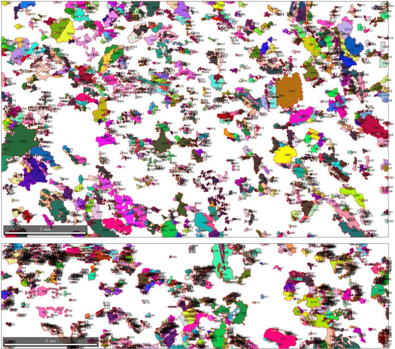
Figure 3 Orientation map of plagioclase grains within Westerly Granite sample.
