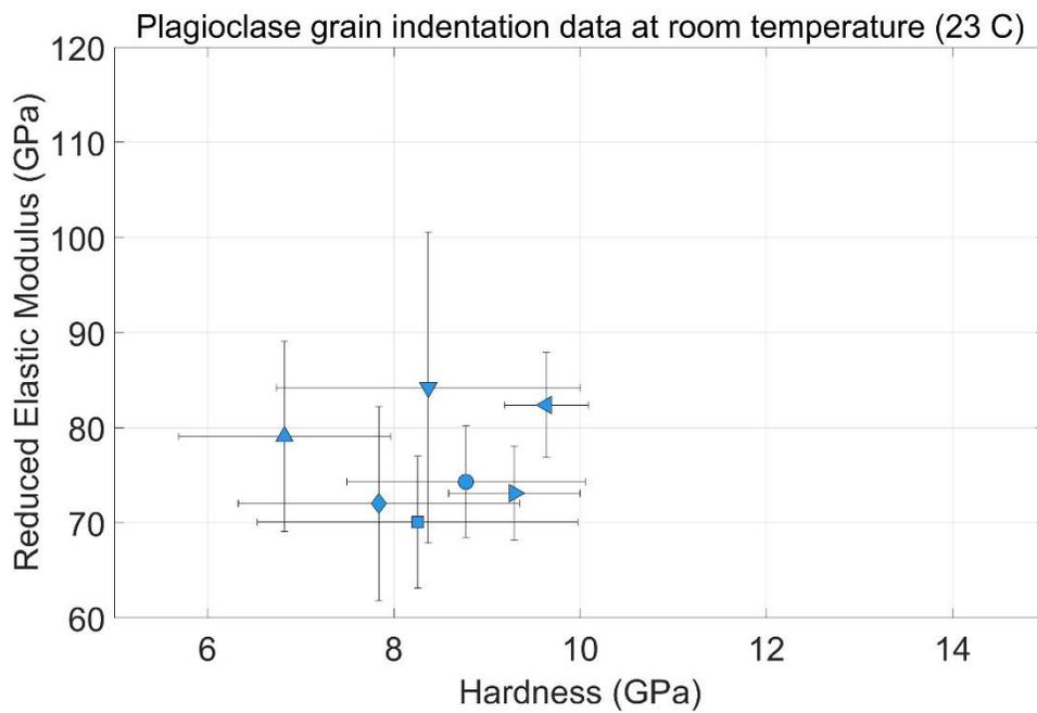
**Figure 10** Average elastic modulus vs. average hardness for all plagioclase grains tested at room temperature.
