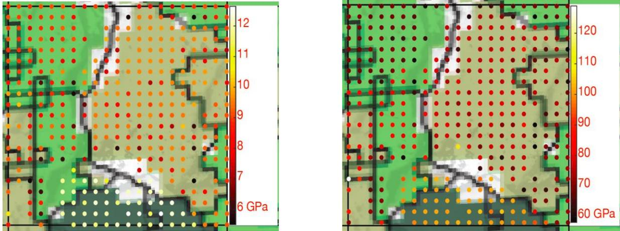
Figure 7 Hardness (left) and elastic modulus (right) of 21x21 indentation array area with 20  $\mu\text{m}$  spacing.
