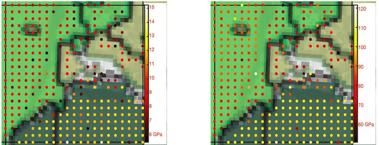
*Figure 6* Hardness (left) and elastic modulus (right) of a different 21x21 indentation array area with 10  $\mu\text{m}$  spacing.
