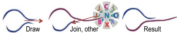
Figure 3: The user drew a stroke that the system assigned to the wrong curve. The user over-rides that choice by tapping on the end of the stroke, which brings up the stroke menu. The user can pen-down on the “join” option and draw to the desired curve. Menu options, from top clock-wise: Combine two curves, Smooth the join, Oversketch, New closed curve, Delete, Back-and-forth scratch, Join, Join and close. Center option is for New curve.
