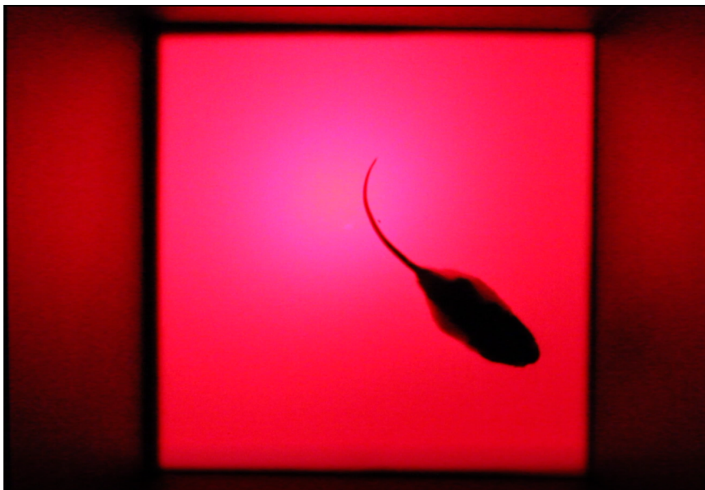
Figure 1: A rodent stands on top of the backlit red acrylic sheet to create a silhouette effect. This light-dark difference makes gray-scale thresholding easier and more reliable.
