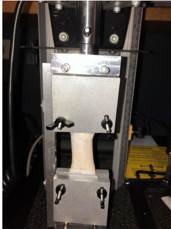
Figure 2: The final clamp design used for all preliminary, current, and future testing. On the left side of the clamps, there is a support bar in order to maintain a constant gauge length. The middle square pieces clamp the tendon.
