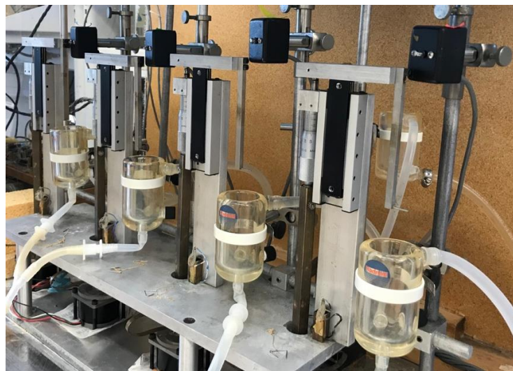
Fig. 2 Image of four load cells without the wires and Arabidopsis hypocotyls attached.
