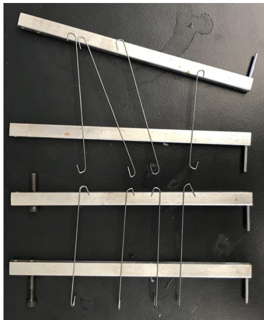
Fig. 3 Image of eight steel wires: four wires with hooks in parallel and four with hooks in a perpendicular orientation
