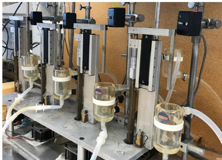
**Fig. 2 Image of four load cells without the wires and Arabidopsis hypocotyls attached.**
