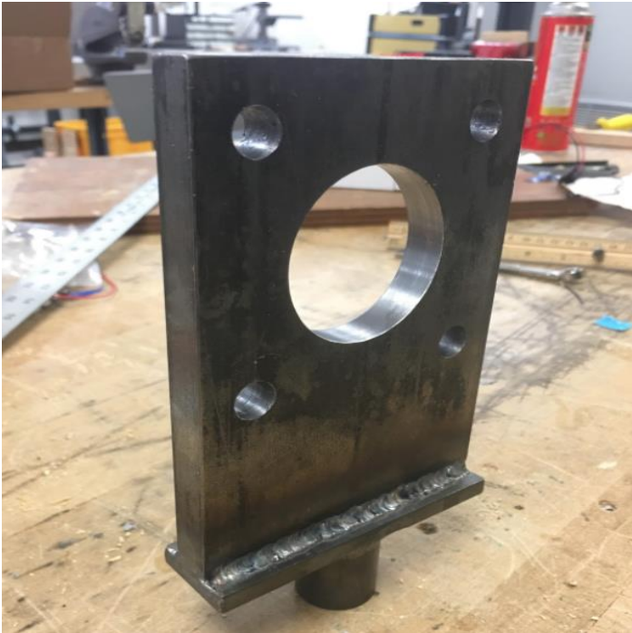
Figure 28 – Bottle jack attachment for front support
