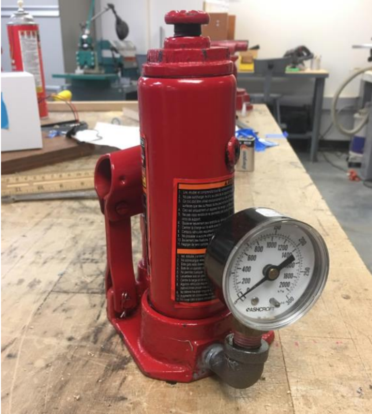
Figure 27 – Modified bottle jack with pressure gauge to measure the applied force to the chassis
