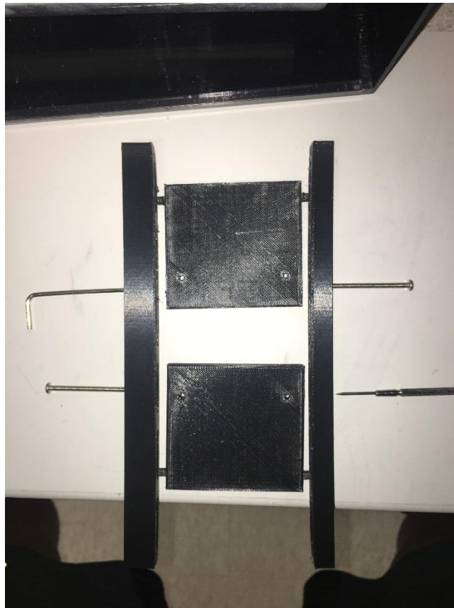
Figure 3: 3D printed prototype clamps
