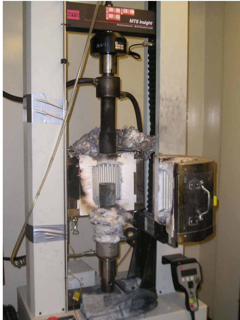
Figure 4.4 Experimental set-up for isothermal high-temperature compression testing of TNZT alloys
