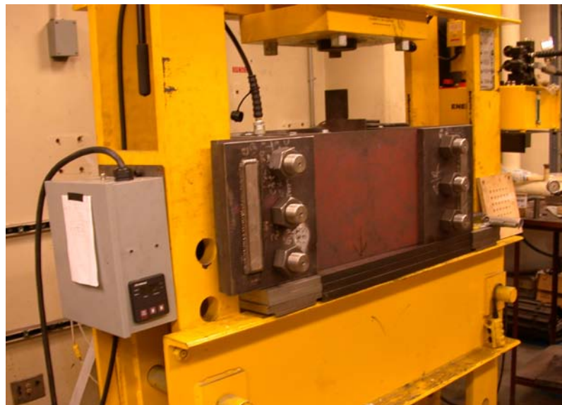
Figure 6.8 Fully assembled ECAE scale-up workstation
