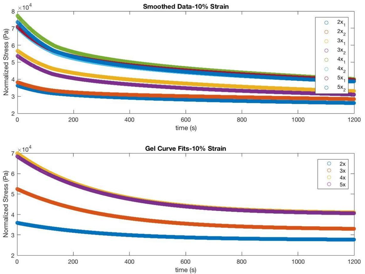
**Figure 6- Smoothed Stress Relaxation data (top) and stress relaxation curve fits (bottom). The graphs show that an increase in the amount of alginate used leads to a higher initial elastic response. This is not true when comparing the 4x and the 5x gels leading to the idea that gel strength may reach an asymptote when compared to increasing amounts of alginate used.**
