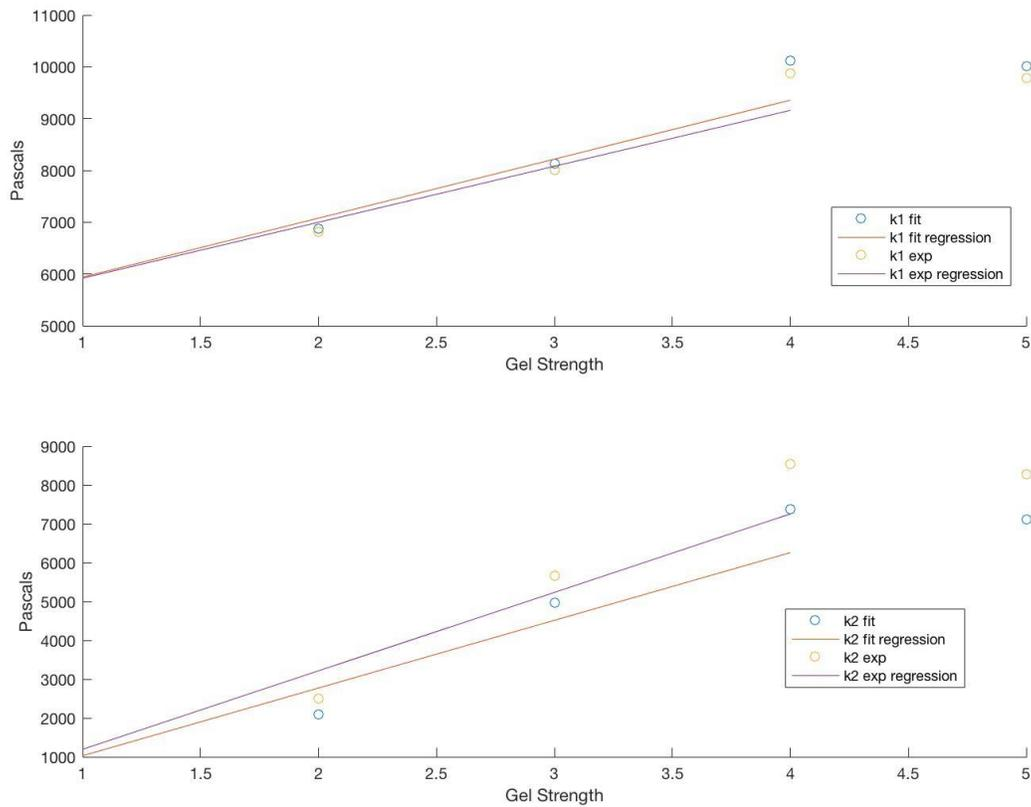
**Figure 8- Linear fits of the  $G_1$  and  $G_2$  (labelled  $k_1$  and  $k_2$  on the legend). The strength of the gels seems to increase linearly except for the x5 gel which does not seem to follow the pattern.**
