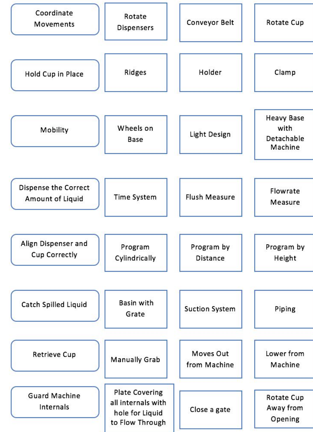
Figure 2: Morphological chart for automated color selector
