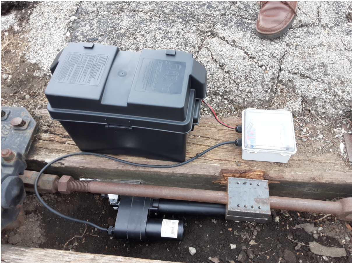
FIGURE 26: REMOTE RAIL SWITCH FULL ASSEMBLY.
