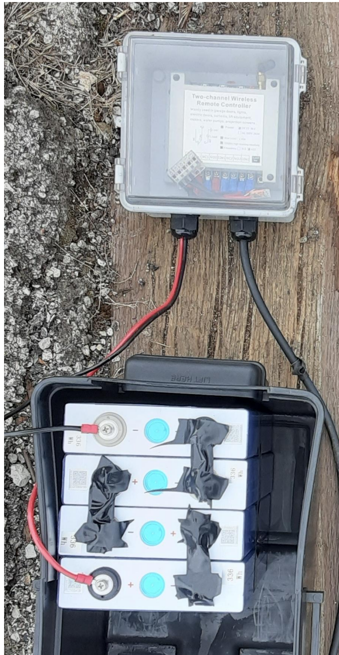
FIGURE 31: BATTERY AND RF CONTROLLER.
