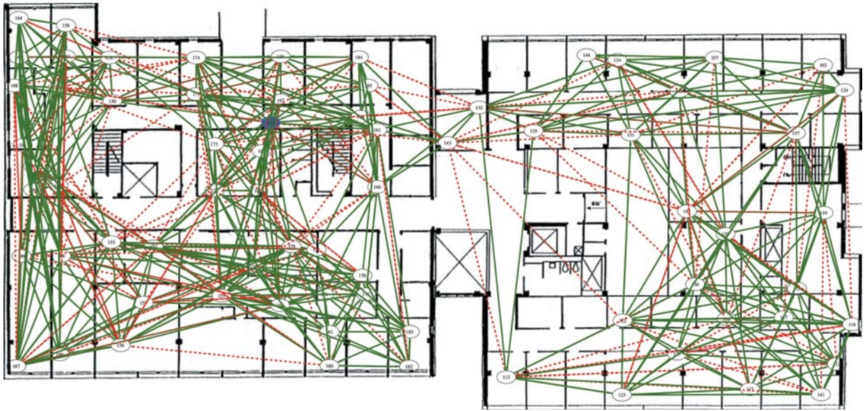
Fig. 5. Testbed topology at -5 dBm Tx power (solid green lines are communication link; dotted red lines are interference link; the sink is colored in blue)
